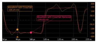
Determine the effects of aggressors on a signal before you do the design work to remove them using the exclusive crosstalk analysis application (D9020ASIA).
