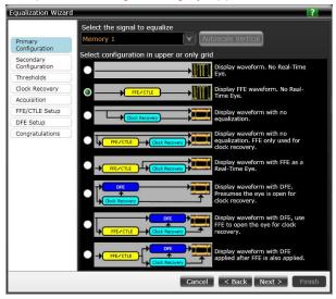
Setup wizards, exclusive to Infiniium, walk you step-by-step through every setting you need to adjust for the best measurements. This equalization wizard helps you open closed eyes on fast data streams using proprietary techniques to remove effects of cables, probes or fixtures from your measurement.
