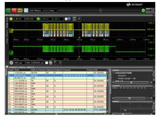
Use one of Keysight's protocol decoding and triggering application packages for increased productivity. The software converts DSO or MSO physical layer acquisitions into packets for specific protocols. Only Keysight offers this breadth, with over 30 protocols available.
