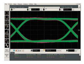
The industry's flattest frequency response leads to excellent correlation between scope only (green trace) and scope plus probe (red trace) measurements as shown in this dual infinite persistence eye diagram.
