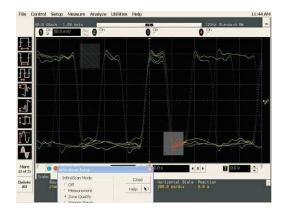
The "true" ease of use. Just draw boxes and the scope will trigger. The industry's only software event finder, InfiniiScan event identification tool provides the next level of ease of use for the scope triggering system.
