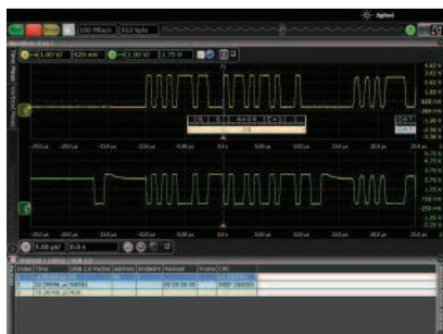
Trigger on and decode USB packets.
