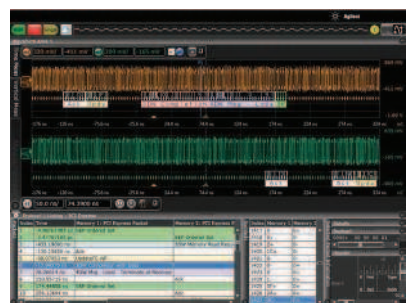
Trigger on and decode PCIe serial packets.
