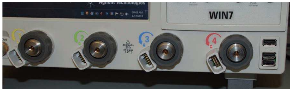
Figure 3 90000 X-Series Oscilloscope Probe Connectors
