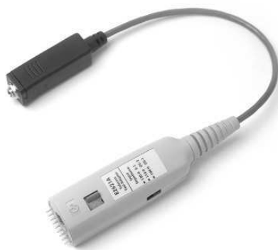
Figure 5. The Agilent E2621A ac-coupled, balanced adapter allows connection to differential communications signals by terminating the signal into 100, 110, or 120 ohms.
