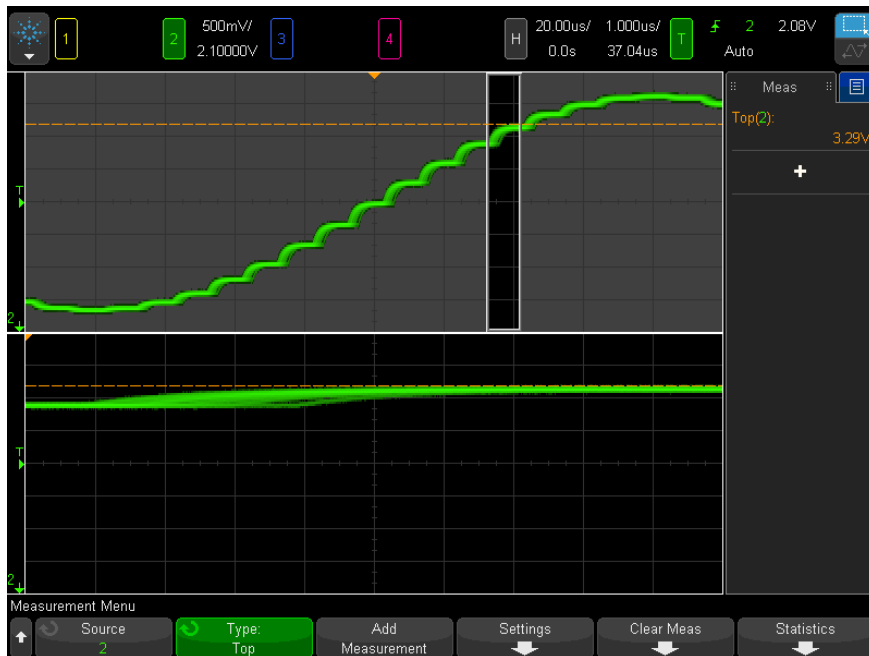
Figure 47 Isolating area for Top measurement
