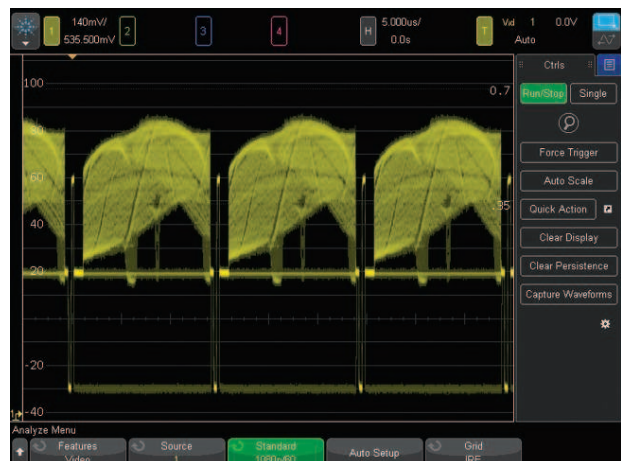
Figure 26: Triggering on 1080p HDTV signal analysis.
