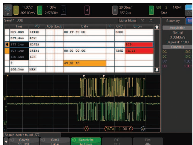
Figure 20: USB 2.0 trigger, decode and "lister" display.
