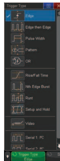
Figure 42: Wide array of advanced parametric trigger modes.
