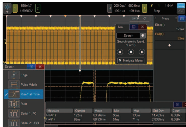
Figure 10: The 4000 X-Series was set up to capture data signals with various rise time edges. Using the search and navigation capability, the oscilloscope was able to find, mark (white triangles), and quickly navigate to 16 occurrences of "out of compliance" rise-time edges.
