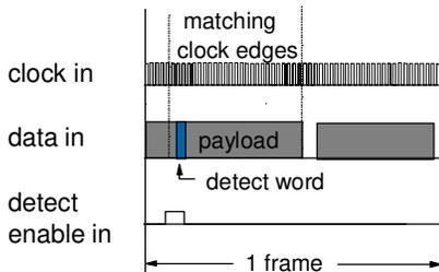
Figure 10: Input signals in cell detect mode
