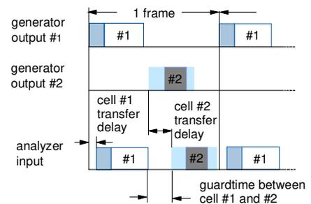
**Figure 7: Timing relations between generators and analyzers**
