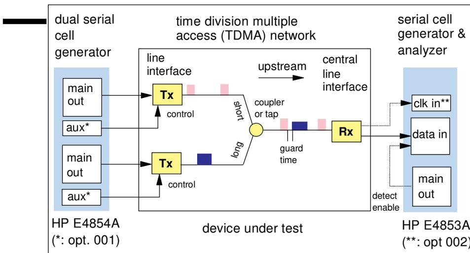
Figure 1: Test set-up for characterizing TDMA devices
