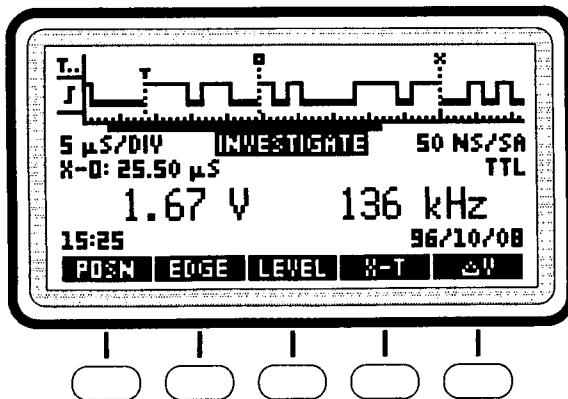
Press the menu key below the label to perform that action. In the display above, pressing the right hand menu key, labeled  $\Delta V$ , turns on or off the  $\Delta V$  measurement (described on page 10).
