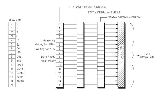
Bits in the Operational Status condition register are set to 1 under the following conditions:
