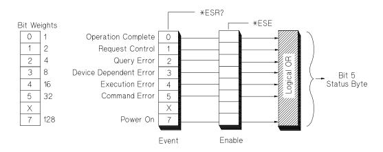
The Standard Event register set does not conform to the general status register model described at the beginning of this chapter. It contains only two registers: the Standard Event event register and the Standard Event enable register.
