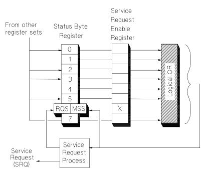
When a register set causes its summary bit in the Status Bytebyte register; description to change from 0 to 1, the module can initiate the service request (SRQ) process. However, the process is only initiated if both of the following conditions are true:
