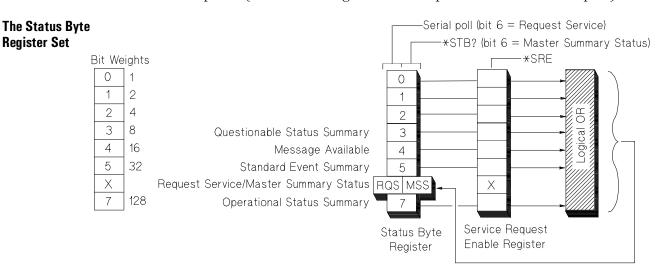
The Status Byte register set does not conform to the general status register model described at the beginning of this chapter. It contains only two registers: the Status Byte register and the Service Request enable register. The Status Byte register behaves like a condition register for all bits except bit 6. The Service Request enable register behaves like a standard enable register except that bit 6 is always set to 0.
