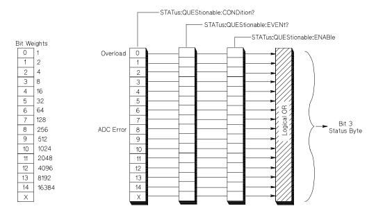
Bits in the Questionable Status condition register are set to 1 under the following conditions.
