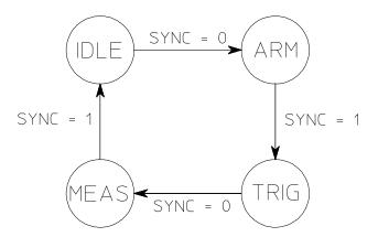
**IDLE STATE** In the idle state the ADC, zoom, and digital filters operate according to their own control registers and according to the OPCODE in the Measurement Control register. No new data is written into the FIFO. Data from the FIFO is available (via the backplane or local bus port) as long as there is data available from the previous measurement. The module can be forced to the idle state by writing an OPCODE  $\neq 2$  in the Measurement Control register.
