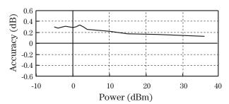
Measurement Frequency is 975 MHz
