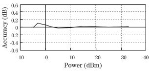
Measurement Frequency is 1880 MHz
