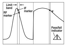
LO alignment is as easy as placing an IF and RF marker within the limit bands. Dual-segment sweeps let you have both a coarse and fine adjustment window for faster alignment.
