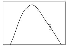
Adjusting and measuring tilt is as simple as ensuring the delta (lower) marker is between the two point limits.
