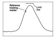
A combination of reference tracking and limit lines let you easily make peak-to-carrier measurements such as peak-to-video, peak-to-audio, and peak-to-color.
