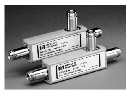
The HP 86205A/86207A high directivity RF Bridges offer unparalleled performance in a variety of general purpose applications. They are ideal for accurate reflection measurements and signal-leveling applications. They combine the directivity and broad-band frequency range of directional bridges and the low insertion loss and flat coupling factor of directional couplers.
