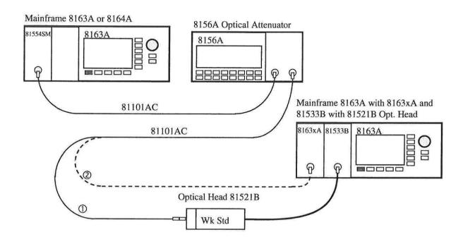
Figure 2 Accuracy Test Setup
