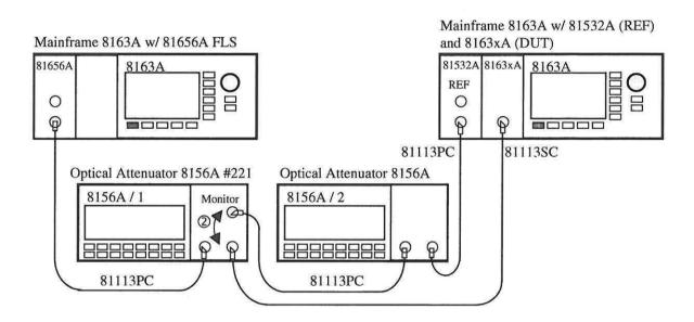
Figure 3 Measurement Setup for Power Linearity
