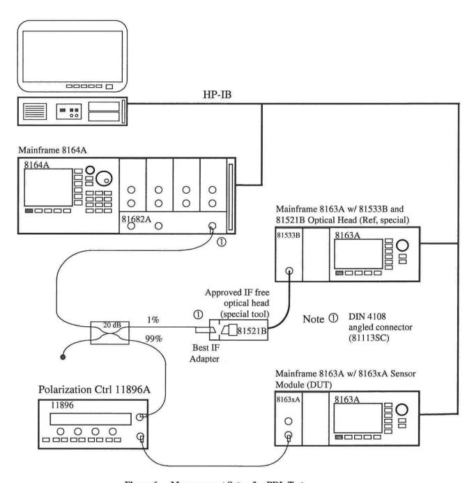
Figure 6 Measurement Setup for PDL Test
