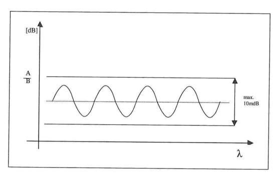
Figure 8 Interference Ripple
