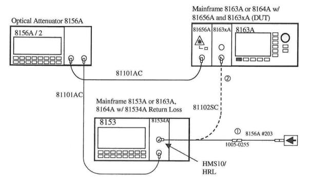
Figure 5 Return Loss Measurement Setup
