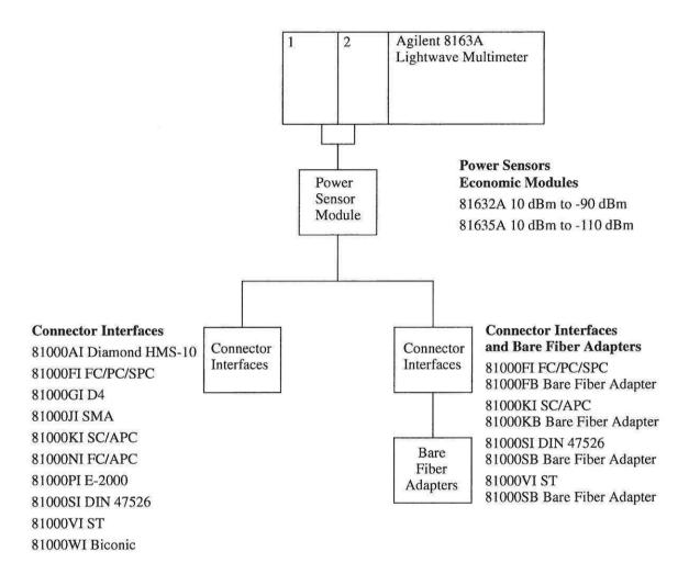
Figure 1 Recommended Connector Interfaces and Bare Fiber Adapters
