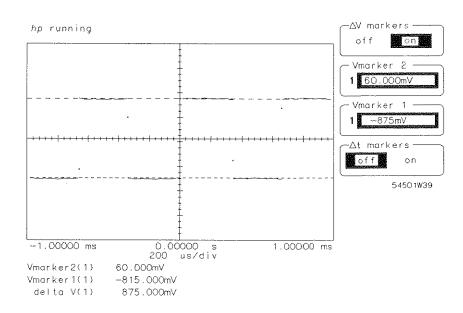
The peak-to-peak value is the *delta* V reading at the bottom of the display.
