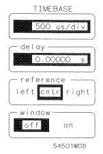
Setting the timebase displays the signal at different time/division settings (Remember the frequency of the HP 54502A is different than the HP 54501A and HP 54503A and will have different values displayed.)
