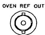
Supplies a 10 \text{ MHz} \pm 1 \times 10^{-7} per month sinusoidal frequency reference from an internal crystal oscillator, located in a temperature-controlled oven. The output is ac coupled and the output impedance is 50 ohms. The nominal output level is +10 dBm/50 ohms. The output is disabled during the oven's warmup cycle. To use the internal Oven Reference, this output must be connected to the EXT REF IN jack.
