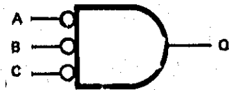
DENOTES "AND" GATE WITH INVERTED INPUTS
