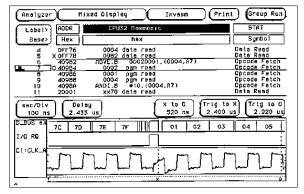
Code listings, timing waveforms, and oscilloscope waveforms can be time-correlated and displayed together to speed troubleshooting.
