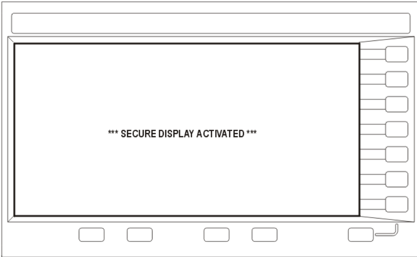
Figure 2-11 PSG Screen with Secure Display Activated
