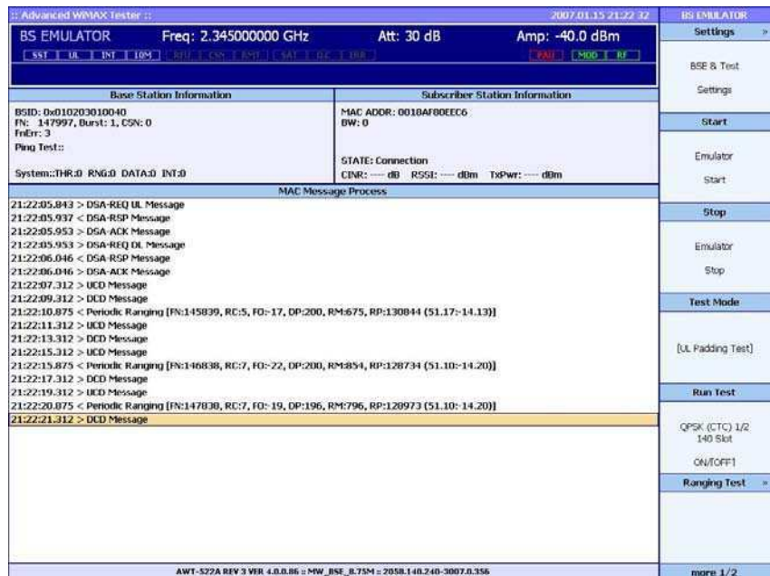
Figure 12 Establishing Two Way Communications Between the E6651A and the SS
