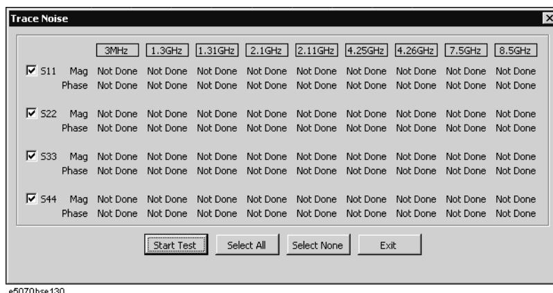
Figure 4-72 Trace Noise tests dialog box example (E5071A)
