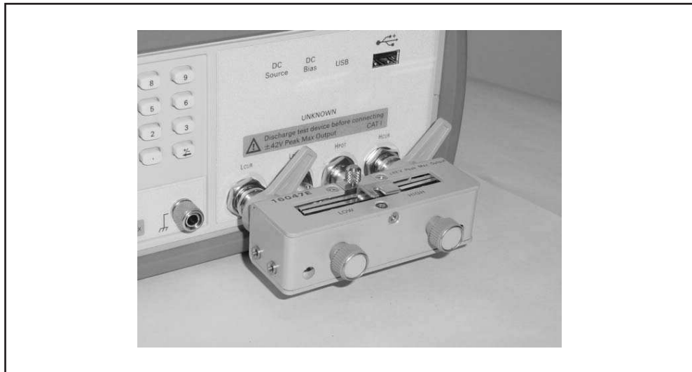
Figure 7-19 Connecting a shorting bar
