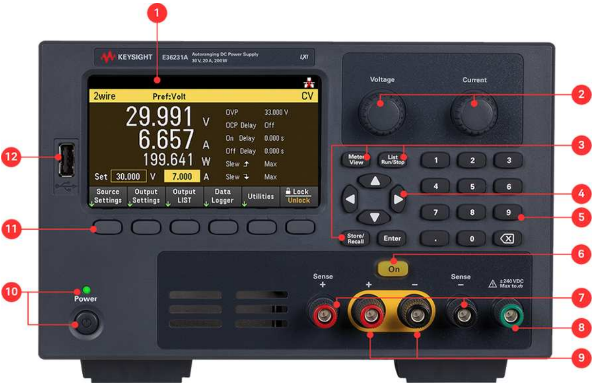
Front panel at a glance (E36231A/E36232A)
