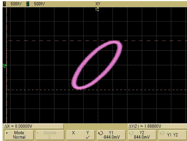
Figure 23 Cursors set on displayed signal
