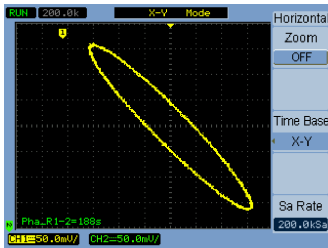
Figure 15 X-Y Display Format Showing Out-of-Phase Waveforms
