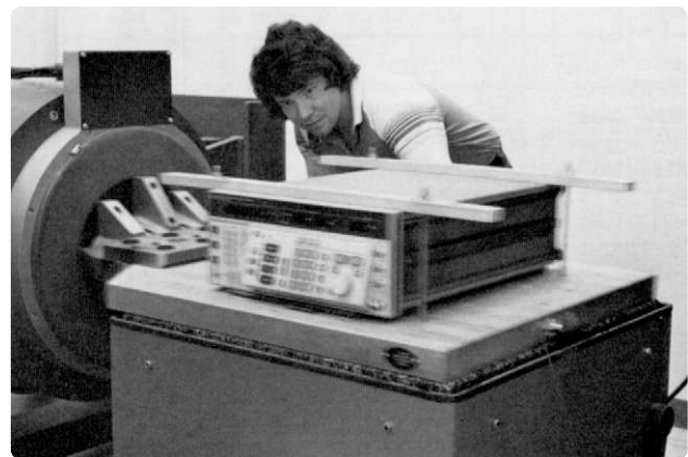
Rigorous type-testing of the 8663A.
