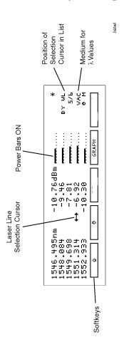
Display after the front-panel Run key is pressed.
