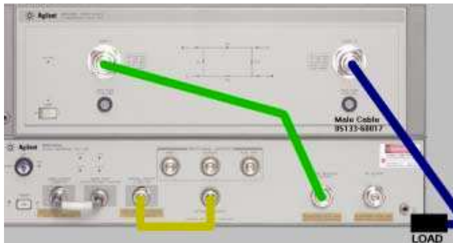
Figure 4-19. Connections for O/E Response and Match Calibration (Std9)
