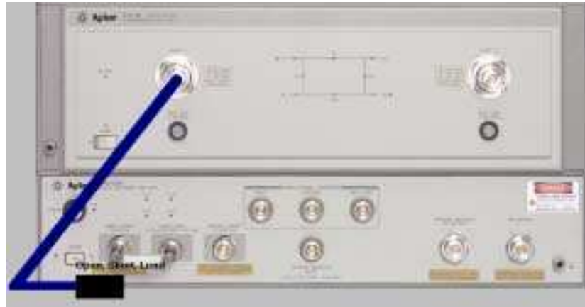
Figure 4-24. Connections for E/O Reflection Response Calibration (Std1, Std2, Std3, Std4), and E/O Bandwidth Reflection Response Calibration (Std1, Std2, Std3, Std4), and E/O Bandwidth Reflection Response & Isolation Calibration (Std1, Std2, Std3, Std4)
