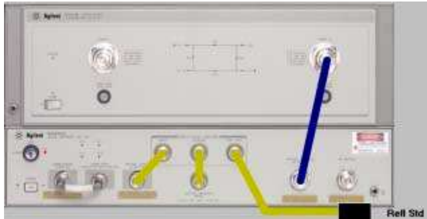
Figure 4-11. Connections for O/E Reflection Response Calibration (Std1), and O/E Reflection Response and Isolation Calibration (Std1, Std2)
