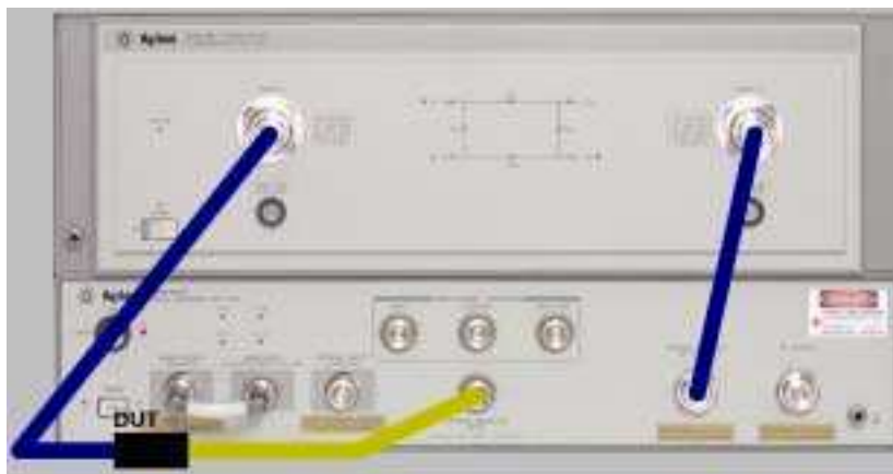
Figure 4-25. Measurement Connections for a Device Under Test after an E/O Reflection Response Calibration
