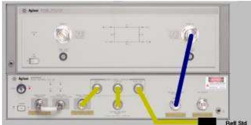
Figure 4-5. Connections for O/O Reflection Response Calibration (Std1), and O/O Reflection Response Calibration (Std1, Std2)
