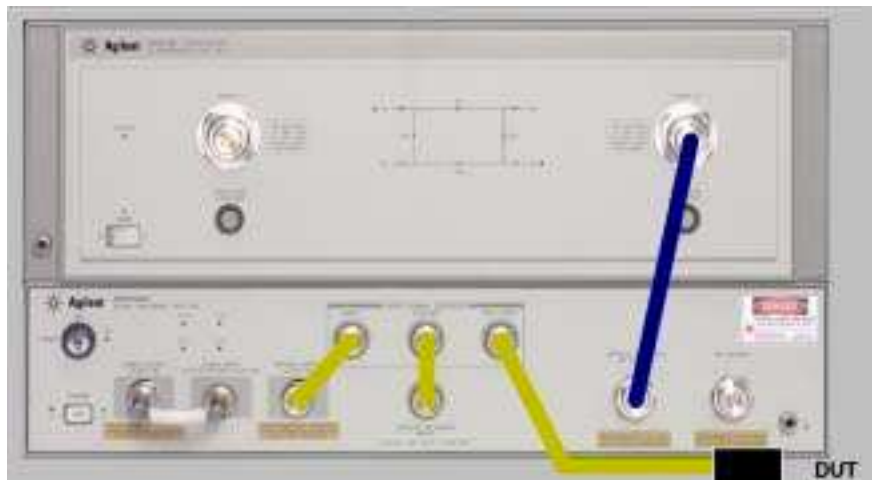
Figure 4-6. Measurement Connections for a Device Under Test after an O/O Reflection Response Calibration
