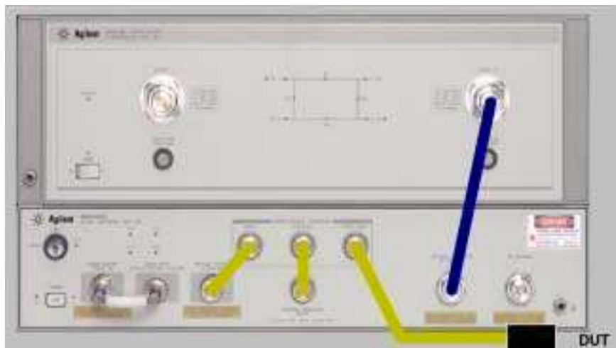
Figure 4-7. Measurement Connections for a Device Under Test after an O/O Reflection Response and Isolation Calibration
