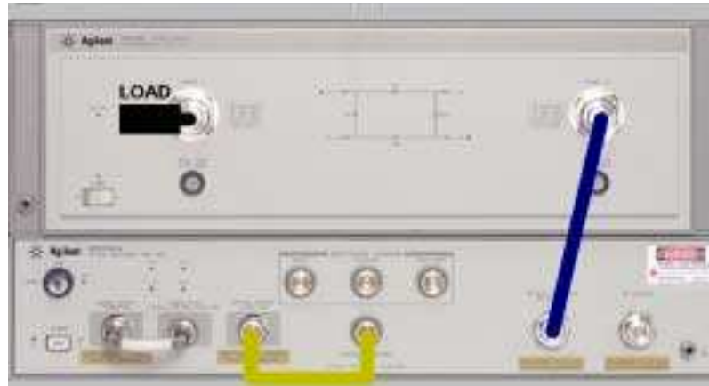
Figure 4-3. Connections for O/O Bandwidth Response (Std1), and O/O Bandwidth Response and Isolation (Std1, Std2)
