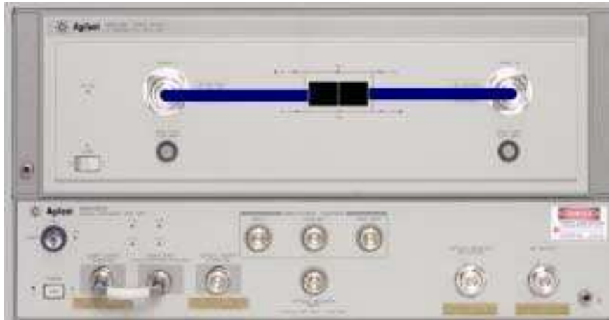
Figure 4-26. Connections for E/O Bandwidth Reflection Response Calibration (Std5), and E/O Bandwidth Reflection Response & Isolation Calibration (Std5)
