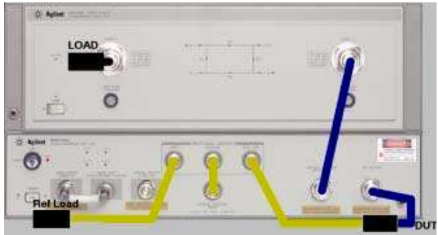
Figure 4-28. Connection for E/O Reflection Sensitivity Calibration (Std1)
