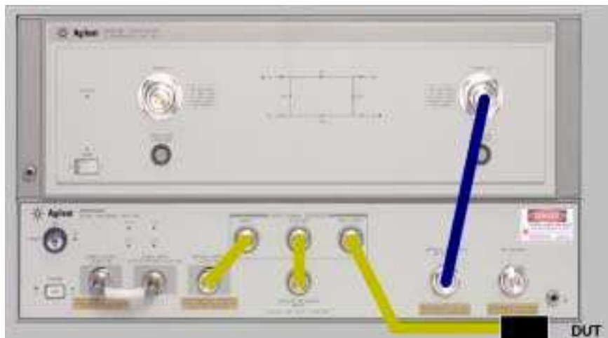
Figure 4-12. Measurement Connections for a Device Under Test after an O/E Reflection Response Calibration or an O/E Reflection Response & Isolation Calibration
