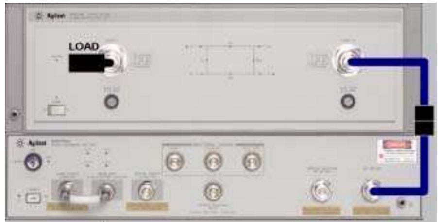
Figure 4-21. Connections for E/O Bandwidth Response Calibration (Std1), and E/O Bandwidth Response & Isolation Calibration (Std1)
