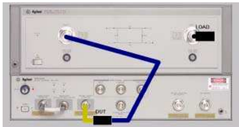
Figure 4-9. Measurement Connections for a Device Under Test after an O/E Bandwidth Response Calibration
