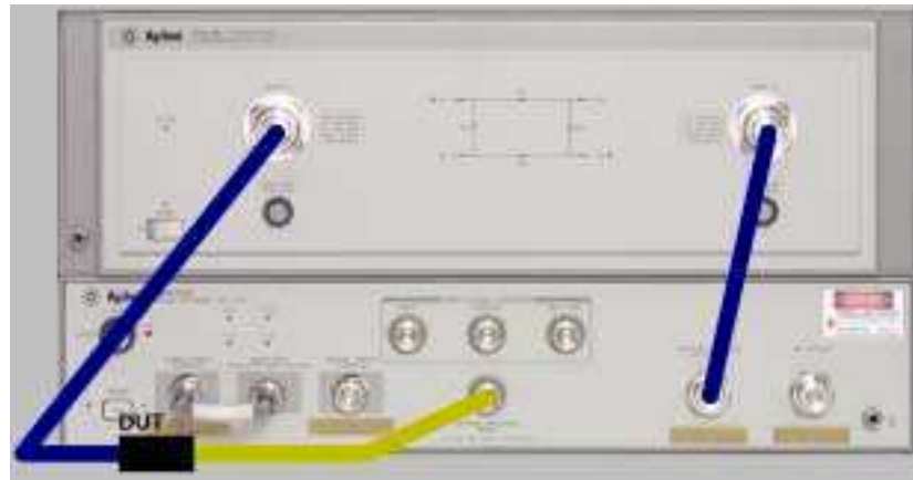
Figure 4-27. Measurement Connections for a Device Under Test after an E/O Bandwidth Reflection Response Calibration
