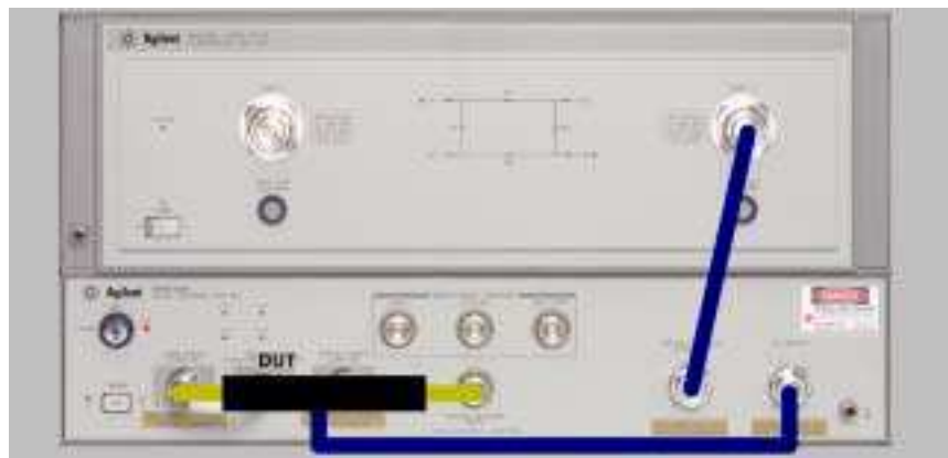
Figure 4-22. Measurement Connections for a Device Under Test after an E/O Bandwidth Response Calibration or an E/O Bandwidth Response & Isolation Calibration
