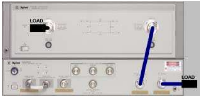
Figure 4-23. Connections for E/O Bandwidth Response and Isolation Calibration (Std2), and E/O Bandwidth Reflection Response and Isolation Calibration (Std6)
