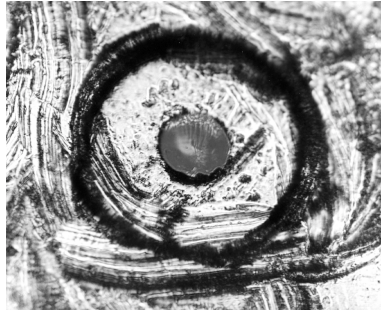
Figure 3-7. Damage from improper cleaning.
