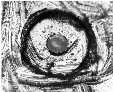
Figure 5-6. Damage from improper cleaning.
