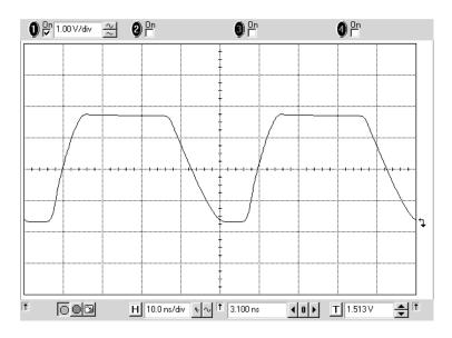
Here is the figure as displayed on the Agilent 54810A Infinium oscilloscope. Use the generator's TRIGGER OUT to trigger the scope.
