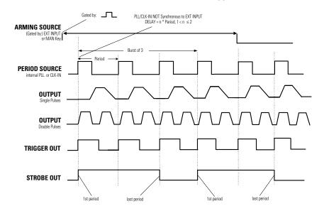
For the second example, either the internal PLL or an external CLK-IN are used to source the period—both cannot be triggered synchronously.
