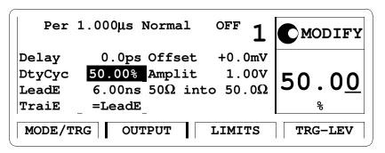
If you need to specify a unit for a parameter, simply press the appropriate unit key (NANO, MICRO/MEGA, MILLI/KILO) instead of the ENTER key.
