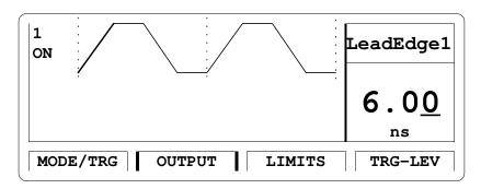
You can modify the parameter displayed in the Modify/Enter area, and immediately check how your changes affect the signal. Use the cursor keys to switch to another parameter.
