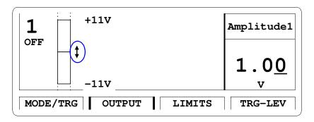
When output limits are on, the limits are indicated on the Output screen in graphics mode (see *"The Limits Screen" on page 64*).
