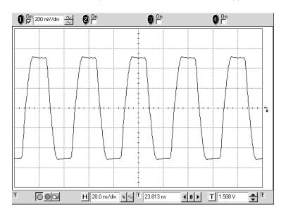
Here is the signal as displayed on an Agilent 54810A Infinium oscilloscope. Use the generator's TRIGGER OUT to trigger the scope.
