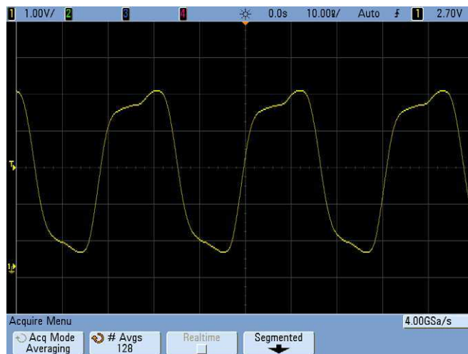
Figure 34 128 Averages used to reduce random noise
