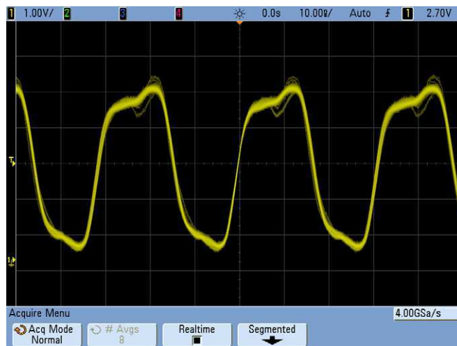
Figure 34 128 Averages used to reduce random noise
