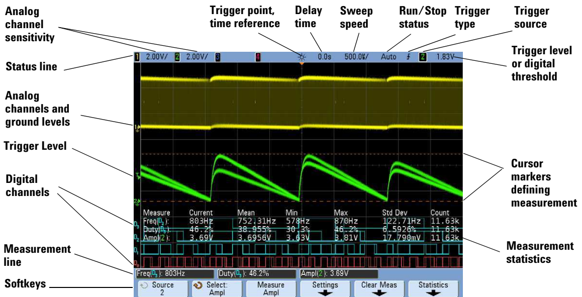
Figure 1 Interpreting the oscilloscope display
