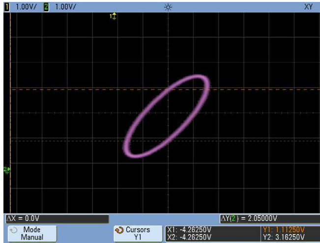
Figure 5 Cursors set to center of signal
