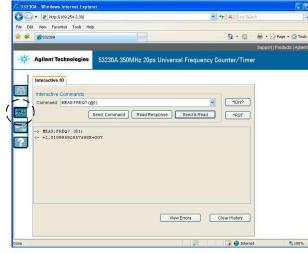
Enter commands from the counter's SCPI command set using the 'Command' window. Query commands which include '?' return data and can be sent using Send & Read. Commands which do not return data are sent using Send Command
