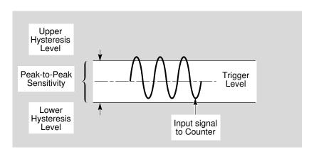
Signal will not generate a count because the trigger level is set below the midpoint of the signal, causing the lower hysteresis level to not be crossed.
