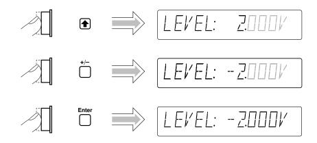
Channel 1's trigger level is now set to -2V.
