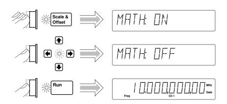
The Counter is now making measurements without the scale/offset values calculated into the measurements.
