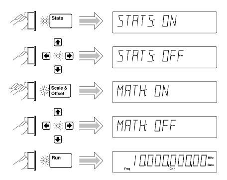
The Counter is now making and displaying normal measurements (that is, the Counter is not showing statistics or scale/offset results).
