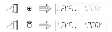
Channel 1's trigger level is now set to +1V.
