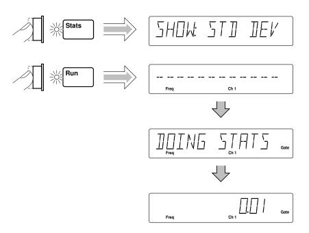
The standard deviation value shown in the previous illustration is for demonstration purposes. The statistic is computed using only those measurements which fell within the limits you set.
