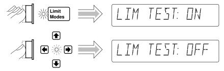
The Counter is now making measurements without limit testing.
