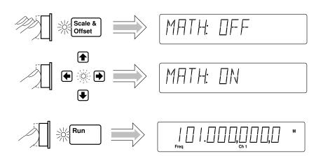
The result of this Math operation is a measurement of 101 MHz.
