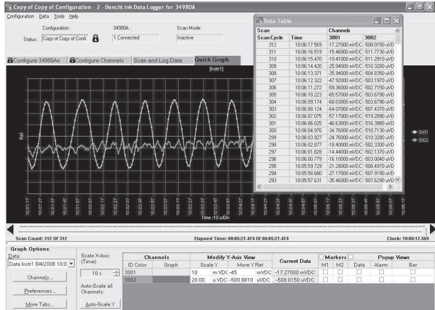
Figure 2. 34826A BenchLink Data Logger Software for high speed data logging with no programming
