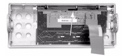
**b** The rubber keypad can now be pulled from the plastic housing.
