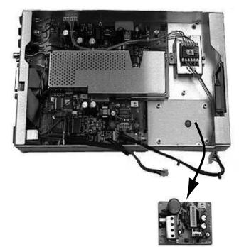
**7 Remove the Power Supply Assembly.** Remove the four Torx screws holding the power supply assembly in place and lift out the power supply.
