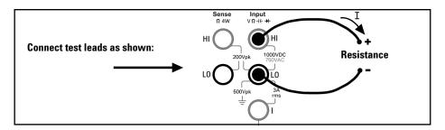
To null-out the test lead resistance:
