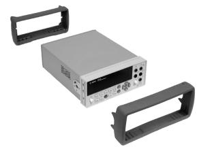
**3 Remove the instrument bumpers**. Pull from a corner and stretch the bumpers off the instrument.
