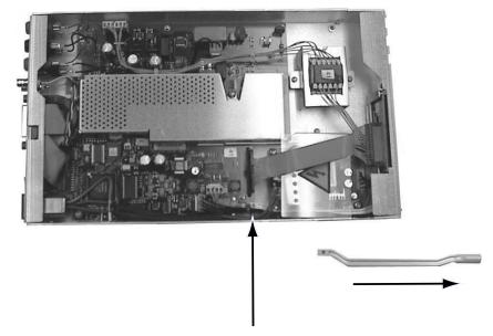
**4 Remove the Display Cable from the main circuit board.** Release the cable connector key from the main circuit board. If desired, remove the display cable by releasing the cable connector key on the *underside* of the display assembly.
