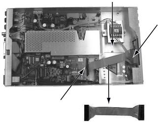
6 Remove the power supply input and output cables.
