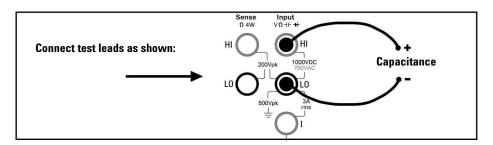
To null-out the test lead capacitance:
