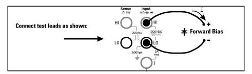
The diode check function is used to indicate correct diode operation; closed-circuit on forward bias and open-circuit on reverse-bias.
