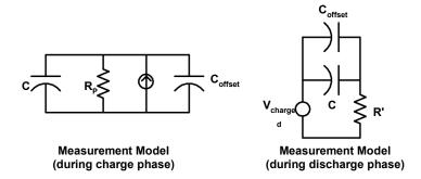
Capacitance is calculated by measuring the change in voltage ( $\Delta V$ ) that occurs over a "short aperture" time, ( $\Delta t$ ). The measurement cycle consists of two parts: a charge phase and a discharge phase.
