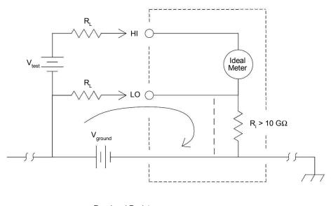
$R_L$  = Lead Resistance  $R_L$  = Multimeter Isolation Resistance  $V_{ground}$  = Voltage Drop on Ground Bus
