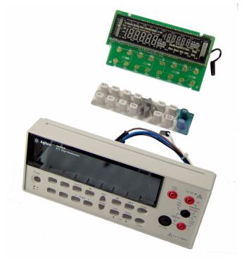
**a** The rubber keypad can now be pulled from the plastic housing.
