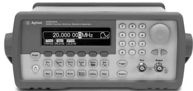
numeric keypad can be used to adjust frequency, amplitude, offset, and other parameters. You can even enter voltage values directly in V<sub>pp</sub>, V<sub>rms</sub>, dBm, or as high and low levels. Timing parameters can be entered in Hertz (Hz) or seconds.
