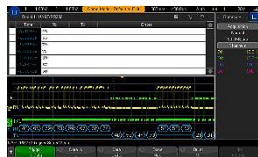
Figure 16. RS232 decode and trigger.
