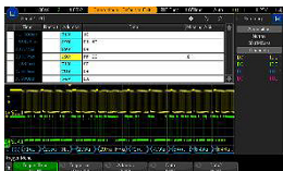
Figure 15. I 2 C decode and trigger.
