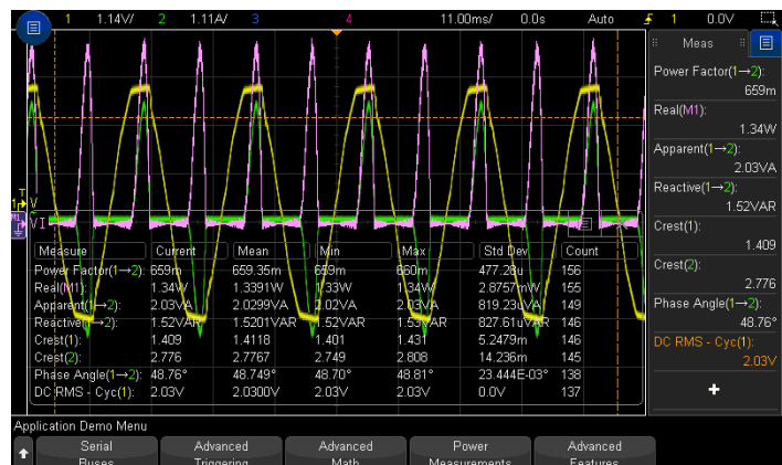
Figure 30a. Integrated power measurements make quick work of analyzing power producing and power consuming devices.
