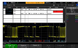
Figure 17. CAN-FD decode and trigger.
