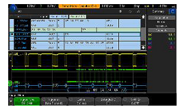
Figure 19. Multi-bus time aligned decode.
