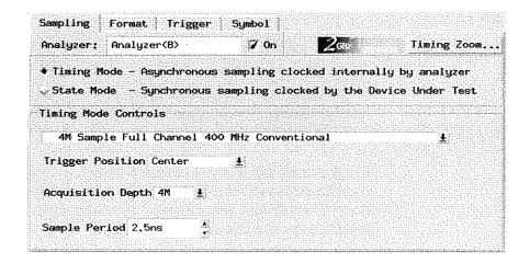
When you select Timing Mode, the Timing Mode Controls area appears.
