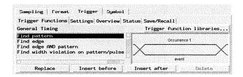
Trigger functions provide a simple way to set up the analyzer to *trigger* on common events and conditions. A library of functions is available for both *state* and *timing* measurements.
