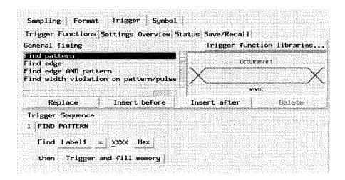
The Trigger tab is used to tell the analyzer when to capture data. The key event is the *trigger*.
