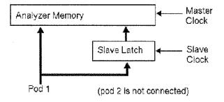
When the slave clock occurs, data captured on the pod is saved into the slave latch for the other pod in the *pod pair*. Then, when the master clock occurs, data captured on the pod, as well as the slave latch data, are saved in logic analyzer memory.
