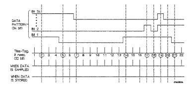
In most cases a transitional timing trace is stored by a mixture of the minimum and maximum cases. Therefore, in this example the actual number of transitions stored will be between 1023 and 2047.
