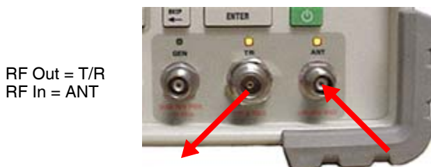
Fig. 3-31 TR/ANT Two Port Duplex Test Setup
