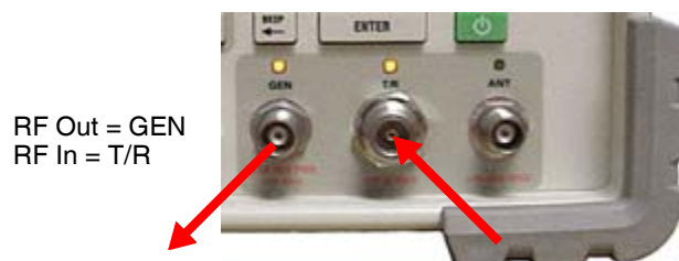
Fig. 3-30 GEN/TR Two Port Duplex Test Setup
