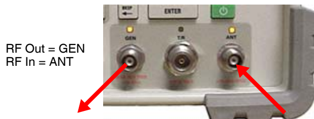
Fig. 3-29 GEN/ANT Two Port Duplex Test Setup
