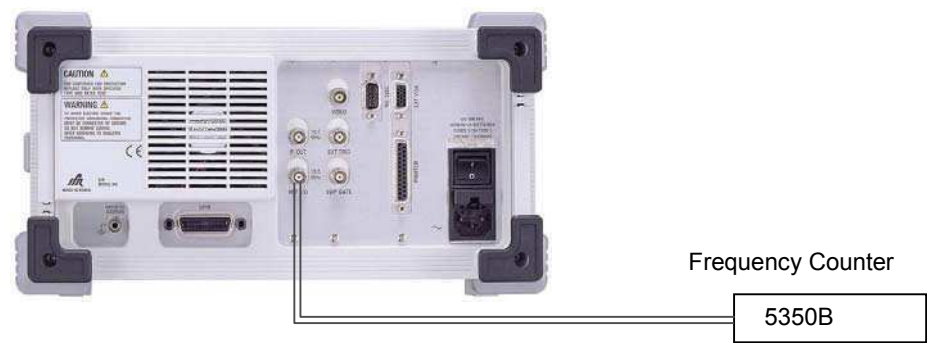
Figure 6-1. Reference Oscillator Frequency Stability Test
