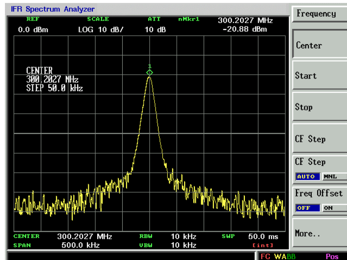
Figure 2-10. Using Signal Tracking to Track a Drifting Signal
