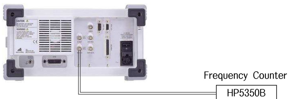
Figure 6-1. Reference Oscillator Frequency Stability Test
