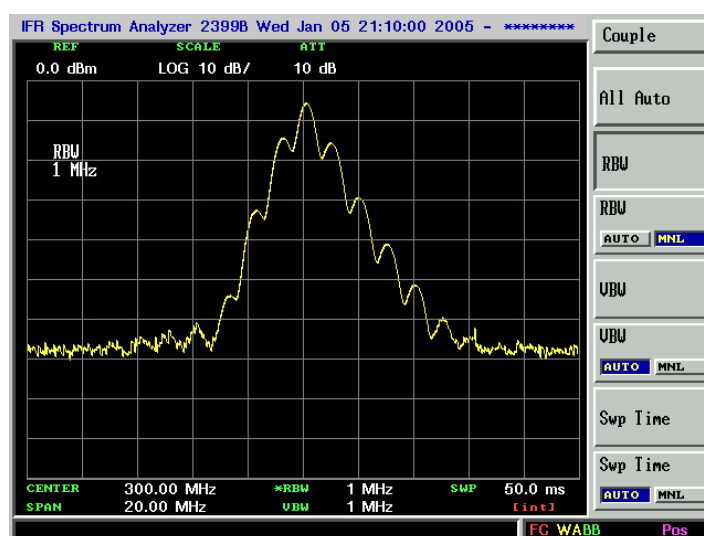
Figure 2-24. Viewing an AM Signal
