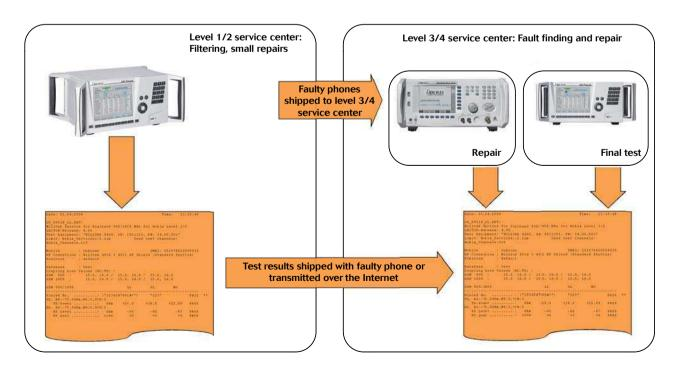
Figure 1: Multi-level repair process
