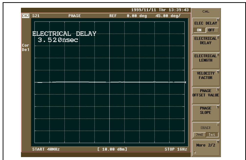
Figure 5-33 Measurement of Electrical Length
