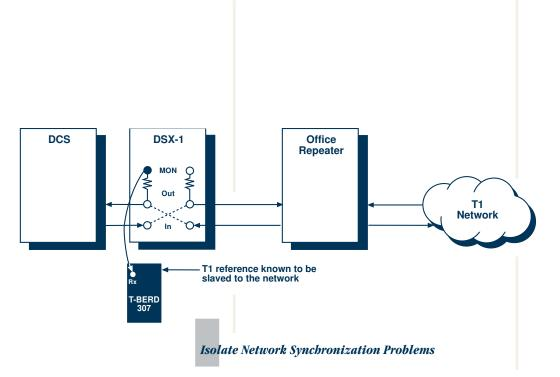
Timing problems are easily identified. Compare T1 circuit against a network reference clock to isolate timing slips.
