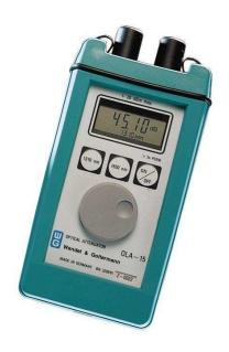
One application of the OLA-15 is in the line-up of optical links, where line interruptions are simulated for bit error testing. The device is also useful when measuring the sensitivity of optical receivers. With its wide variable attenuation range and highly accurate and  $reproducible\ attenuation$ settings, the OLA-15 is an ideal companion for the ONT.
