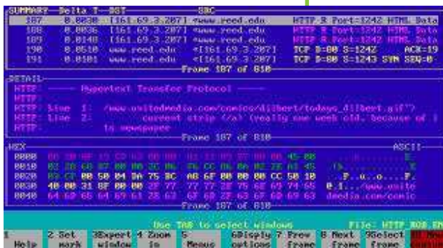
Network General's Sniffer Network Analyzer Option displays LAN decode data in summary, English, and Hex/ASCII formats.
