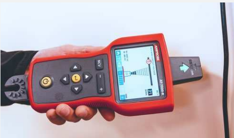
Non-contact voltage (NCV) detection.
