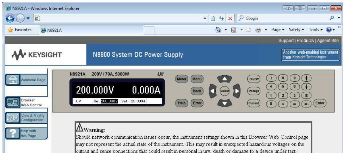
Figure 13. Web graphical user interface for remote access and control of the instrument.
